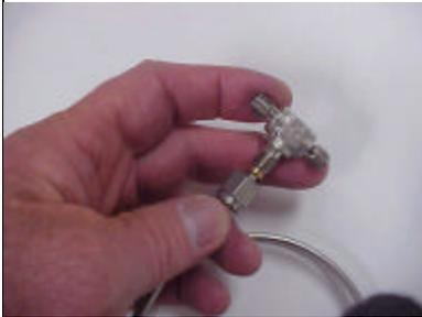
good idea to first tighten the nut and ferrule into a standard swagelok fitting so the ferrule is positioned at a
