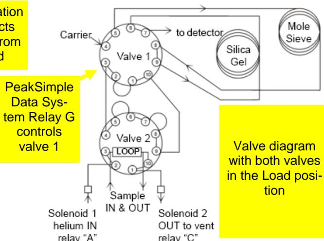
PeakSimple Data System Relay G controls valve 1
