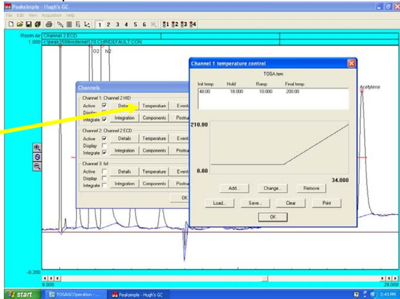
The temperature program should be approximately like the one shown. The initial temperature of 40 degrees should be held constant until the CO peak has eluted and Relay G actuated to return Valve 1 to the LOAD position. The exact timing of this will vary from GC to GC as it depends on the carrier gas flow rate and particular column set installed. See the Multiple Gas #1 instructions for more details on determining the exact timing.
