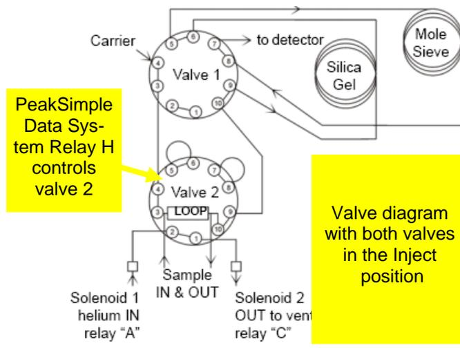
PeakSimple Data System Relay H controls valve 2
