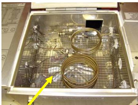
Two 2 meter long packed columns are installed in the GC's column oven, a Silica Gel column and a Molecular Sieve 13X column. The two columns separate the transformer gases in the same way that SRI's Multiple Gas#1 GC configuration does. To understand how the two columns work to perform the separation it would be useful to review the Multiple Gas#1 GC instructions (download from [www.srigc.com](http://www.srigc.com)).
