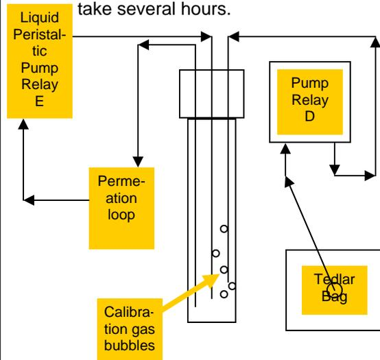
Because the gas is bubbling continuously once the liquid is equilibrated with the calibration gas the concentration of the gas in the liquid does not change further. The liquid can then be used to calibrate the TOGA GC.
