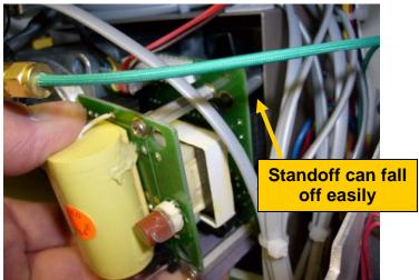
Carefully wiggle out and remove the six pin connector along the top edge of the board. Note that it connects to the leftmost six pins on the board before removing it. Also note the orientation (brown wire on right side).
