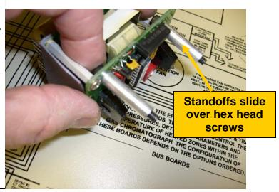
Install the new circuit board set. It is helpful to tilt the board slightly so the standoffs don't fall off while you are wiggling the boards into position.
