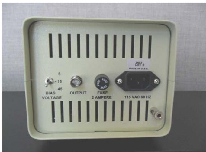
Switch selection of – 5, - 15, - 45 Volt ion source polarization (bias); – 5 V optimum for NP detection, higher polarizations provide 10 times better signal-to-noise for other detection. Twinex connectors on module & accompanying 4 foot long cable provide compatibility for powering ion sources on Agilent, Thermo, Varian/Bruker, and all DET NPD/TID equipment.
