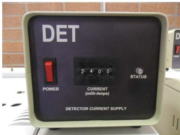
Thumbwheel set of ion source heating current (0 to 4.000 Amps) in 1 mA steps; Red/Green Status Light indicates open circuit or OK in ion source wiring – gives an immediate troubleshooting diagnosis in case of burnout of ion source wire core.
