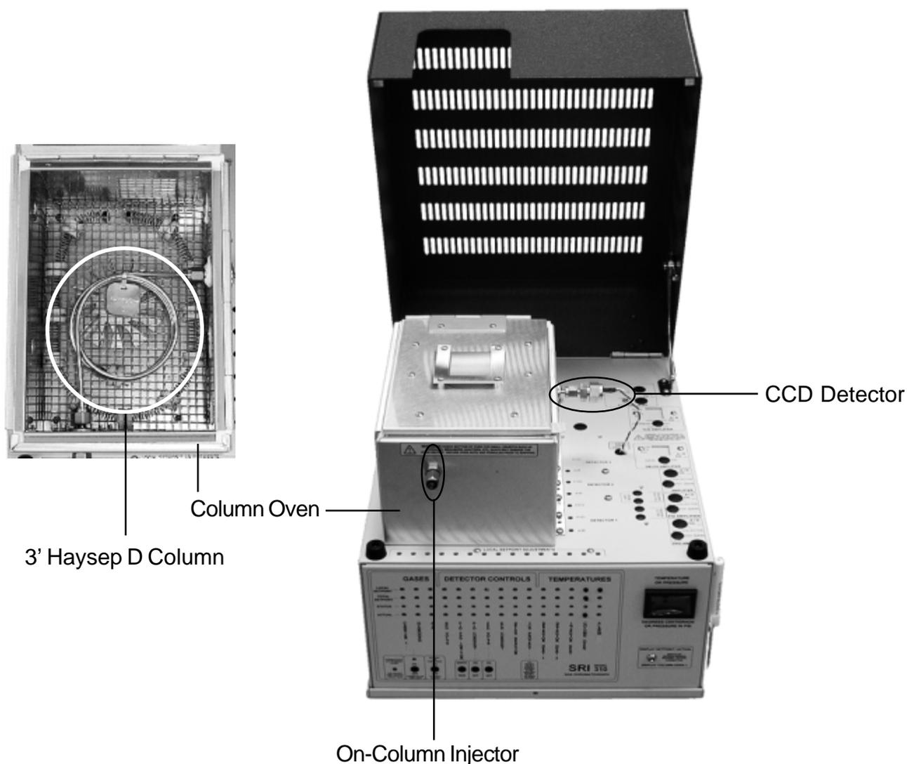
The CCD is about as sensitive as a TCD, but has the hydrocarbon selectivity of an FID. It operates on air alone, which is supplied by the built-in Air Compressor at around 12psi. If you chose optional fast cool-down fans, they will automatically reduce the Column Oven temperature at the end of an analysis to the initial temperature in less than five minutes. Most isothermal applications don't require fast cool-down fans; in these cases, the oven lid is simply manually raised for cooling.
