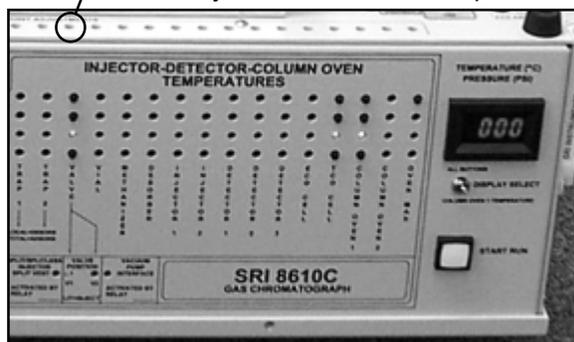
3. Set the valve oven temperature to 90°C using the trimpot on the top edge of the GC front control panel.
