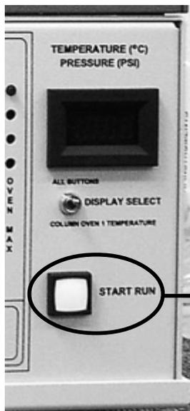
8. Start the analysis by pressing the START RUN button on the front of your GC, or by pressing your computer keyboard spacebar.
