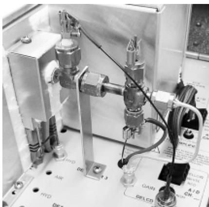
HID detector removed from GC and heater block
