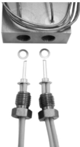
6. Put the new filament's leads through the gland nut. Slide the gland nut up the filament's leads until it rests against the base of the filament. Place the copper gasket against the rim of the detector block cell opening. Carefully insert the filament and gland nut together into the cell opening. Tighten the gland nut to secure the filament in the cell.
