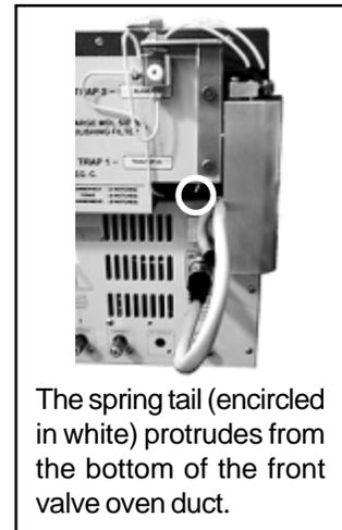
4. To install the 5030 purge head, line up the securing rod with the hole, and gently but firmly push it in until it locks into place. Connect the purge gas in and out lines to the fittings on the top of the front valve oven duct. Connect the dummy 5-pin XLR plug to the socket on the GC.
