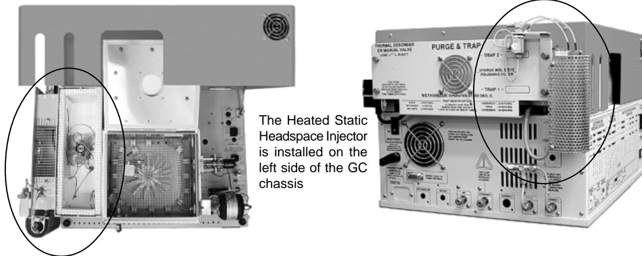
The Heated Static Headspace Injector is installed on the left side of the GC chassis
