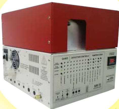
CCD - Detects Hydrocarbons & Hydrogen
