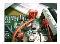
Note that the motor (4 wires-blue, red, green and black) is connected to the bottom of the board on this board variation.
