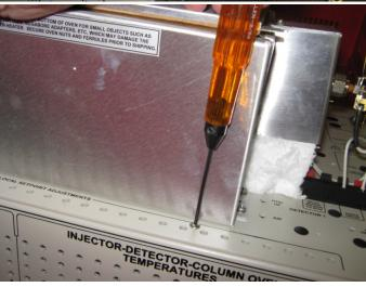
Remove the twelve 1/4inch nuts and lockwashers holding the display board to the front panel.
