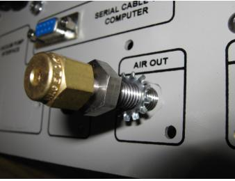
Connect the copper tubing from the filter to the bulkhead fitting on the inside of the chassis.
