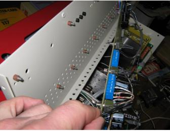
Install the air compressor on/off switch in the circuit board location immediately behind the hole in the front panel.
