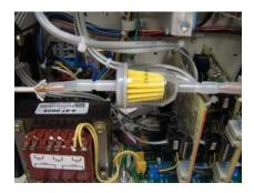
Adjust the filter and tubing so it does not touch any other parts inside the GC.
