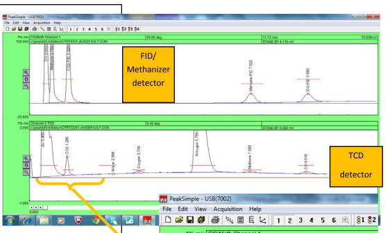
CO2 to methane so the FID/Methanizer can detect those molecules with the same sensitivity as methane and other hydrocarbons. The TCD responds to all molecules including water.
