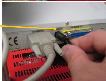
The 24volt power supply is a 50watt (24volts-2.1amps) universal power supply that can work on any line voltage. You may have to change the power plug or cord for your specific country.
