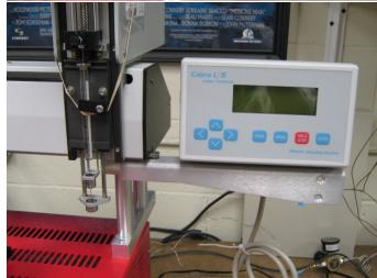
Connect the keypad to the back of the Cobra.
