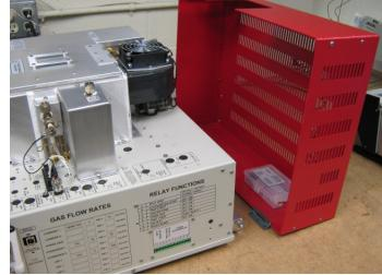
The Cobra should already have the sample vial tray attached. The photo shows the optional 40ml vial (28 vials) tray, but the 2ml vial (120vials) is standard.
