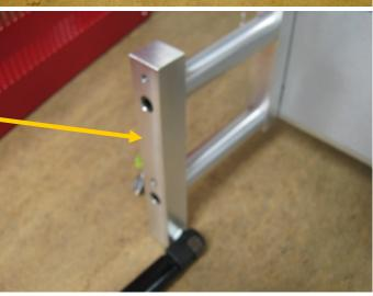
Locate the 4 socket head screws and washers. You will also need a 3/32" hex wrench. A long handled hex wrench makes it easier.
