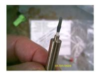
The hydrogen makeup supply can be connected to either restrictor tube. The NPD restrictor tube requires 10psi of H2 pressure to get a flow of 2ml/minute.
