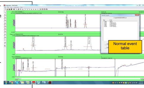
This chromatogram shows the same sample but with Valve 1 and 2 injected simultaneously. Relay A is turned ON at the same time (.1minute) which stops the carrier gas flow in the Haysep and capillary columns. This creates some extra "ghost" peaks but does not substantially affect the analysis. The stop-flow solenoid is turned OFF (reestablishing the flow) at 4minutes.
