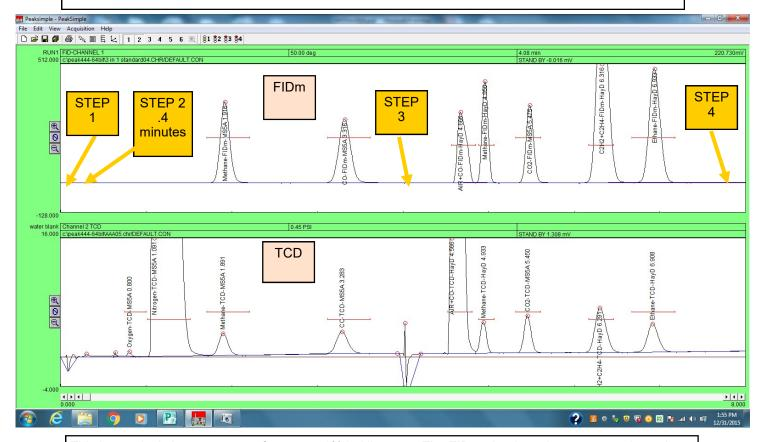
This is a typical chromatogram of gases at 1% in Nitrogen. The FIDmethanizer chromatogram is on the top and the TCD on the bottom.
