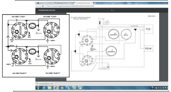
The diagram above shows a schematic of the "basic" MG#5 configuration with both valves in the INJECT position. A similar diagram below shows the "basic" MG#5 plus an additional column and FPD/FID detector to measure sulfur gases like H2S, CO2, SO2, mercaptans, DMS etc.
