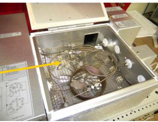
On the right side of the column oven is located the Thermal Conductivity Detector (TCD) which detects all the gases from 200ppm to 100% except hydrogen (see detailed explanation for this later).
