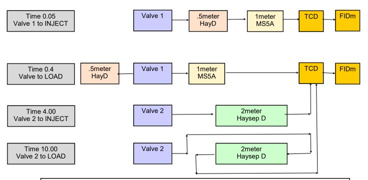
The schematic above shows the 4 steps in the MG5 analysis after the sample has been loaded into the loop of each valve.
