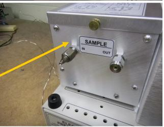
The carrier gas is connected to the left side of the GC. The carrier gas can be helium, hydrogen, nitrogen or argon. Inside the GC there is a very precise pressure regulator called an "Electronic Pressure Controller" (EPC) which supplies the carrier gas at a stable pressure to the valves and columns.
