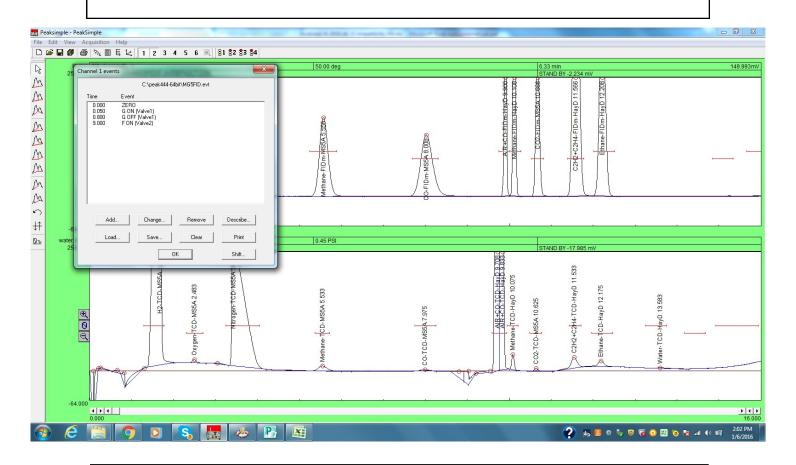
The chromatogram above shows the full analysis including the C2 peaks. Note that the Relay F on time (inject onto the Haysep dolumn) had to be delayed until 9 minutes to allow the CO to elute from the 6'MS5A column before making the injection onto the Haysep column.
