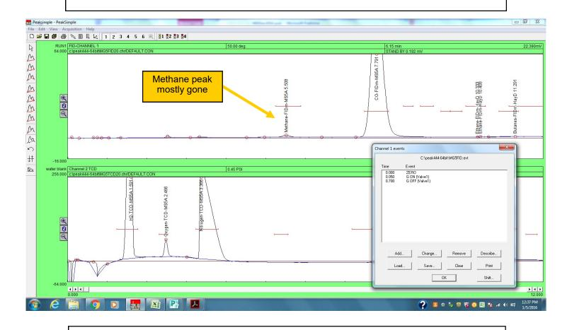
The exact time for Relay G off (backflush pre-column) will be different using Argon vs Helium. By trial and error move the Relay G off time earlier and earlier until you see the methane peak disappear.
