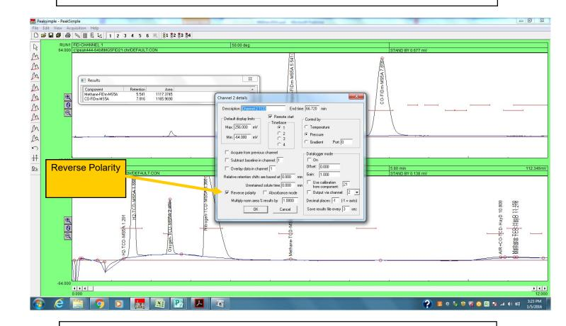
When using Argon or Nitrogen carrier gas the peaks come out upside down. In the channel 2 Details screen, click the box labelled "Reverse Polarity" so the peaks will come out in the positive direction.
