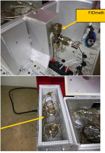
The Valco 10port gas sampling valve (GSV) looks like this. There is an electric motor inside the GC which turns a Teflon seal inside the valve at a specific time during the analysis to change the carrier gas flow path.
