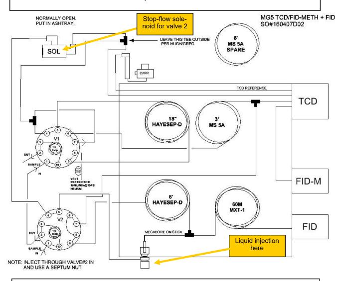
This drawing shows a capillary column and extra FID detector connected at a "tee" fitting so a liquid injection ( or low volume gas injection ) splits onto the capillary and the Haysep column.
