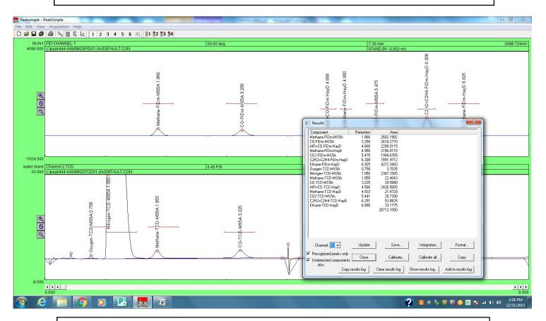
The sample above (helium carrier at 15psi) shows 1% each methane, CO, CO2, ethane, ethylene and acetylene with a little oxygen, and nitrogen balance. Note that the area of the methane, and CO peaks are about the same on the FIDm, and similar but not identical on the TCD.
