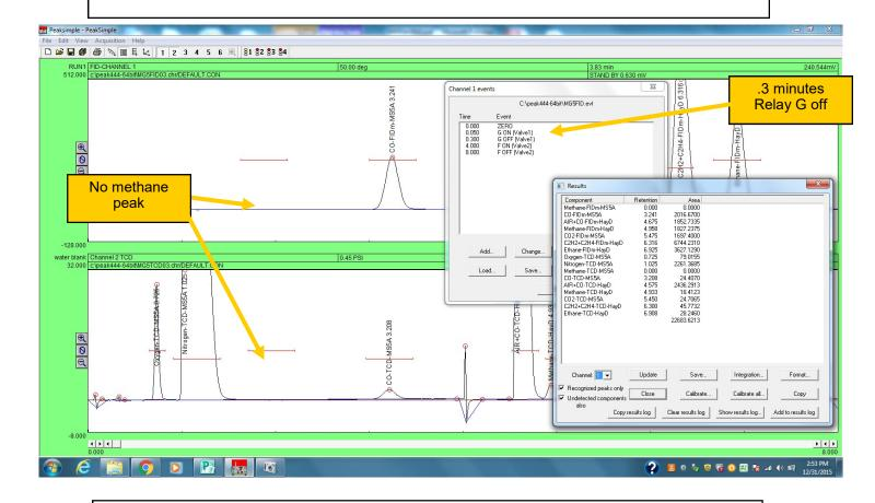
Compare the same sample but with Relay G off at .3 minutes instead of .4 minutes as in the previous page. The methane peak has disappeared because the time that Relay G turned off was too early, so the methane peak did not make it onto the MS5A column and was backflushed off the pre-column ( .5meter HayD ) to vent.
