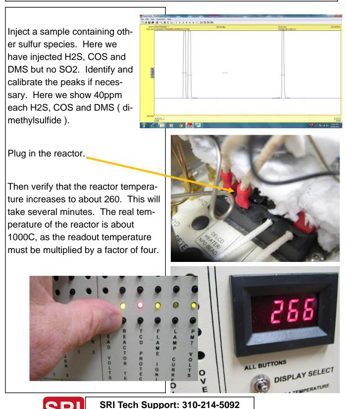
The chromatogram at right shows the same sample (40ppm each H2S, COS and SO2) with the reactor hot (260). The H2S, COS and DMS have all disappeared and a SO2 peak shows instead.
