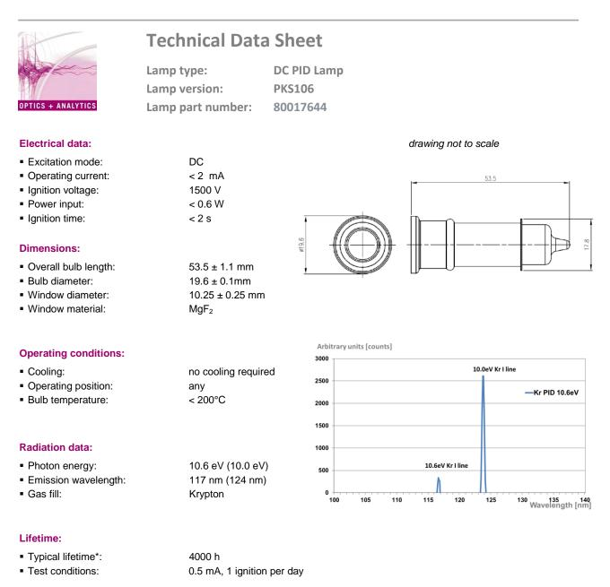
\* The data regarding lifetime have been obtained under continuous laboratory operation on a large numbers of lamps. The typical lifetime set forth above means that radiant power has decreased on average <70% after this lifetime. The actual lifetime of an individual lamp may vary significantly from this value.
