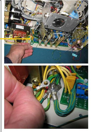
Connect your external device to the relay from the outside of the GC.
