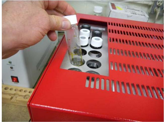
Make a calibration standard for the solvents you want to measure. If the legal limit is 500ppm residual ethanol, then make the standard so the amount of ethanol in the standard is close to what 500ppm ( .05% ) of ethanol would look like if it were in the concentrate.
