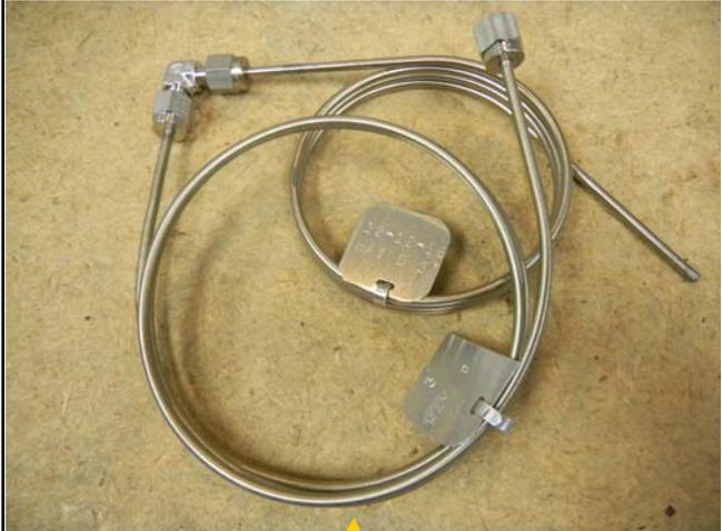
The combo column consisting of a 3 foot Haysep-D and a 3 foot Haysep-R connected in series with a stainless steel fitting can be ordered using SRI part#8600-3D3R which has a list price of \$390 as of January 2017
