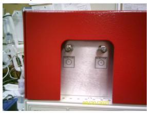
The hydrogen gas produced by the built-in H2 generator is directed to one injector or the other by the two plastic clips
