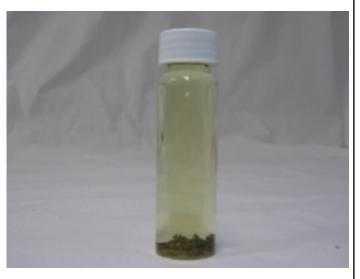
After about 20 minutes, a small amount of the alcohol extract is injected into the GC with a syringe.
